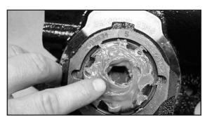
4. Slide the pitman arm puller over the pitman arm as shown. Take care to align the hole in the puller with the Allen socket in the retainer. Insert the Allen drive socket through the puller and into the retainer socket. Use an impact wrench to back off the retainer. The retainer will act as a jack screw to remove the pitman arm.
